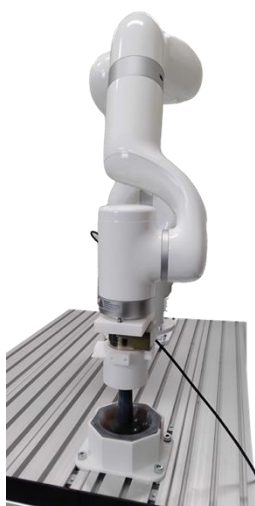
Figure 3. Overview of the automated kneading robot system.
