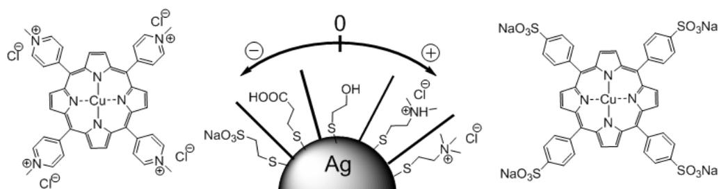
Figure 4. Schematic representation of immobilized Ag NPs surface modification by thiols bearing differently charged functional groups and oppositely charged model analytes CuTMpyP4 and CuTSPP4.
