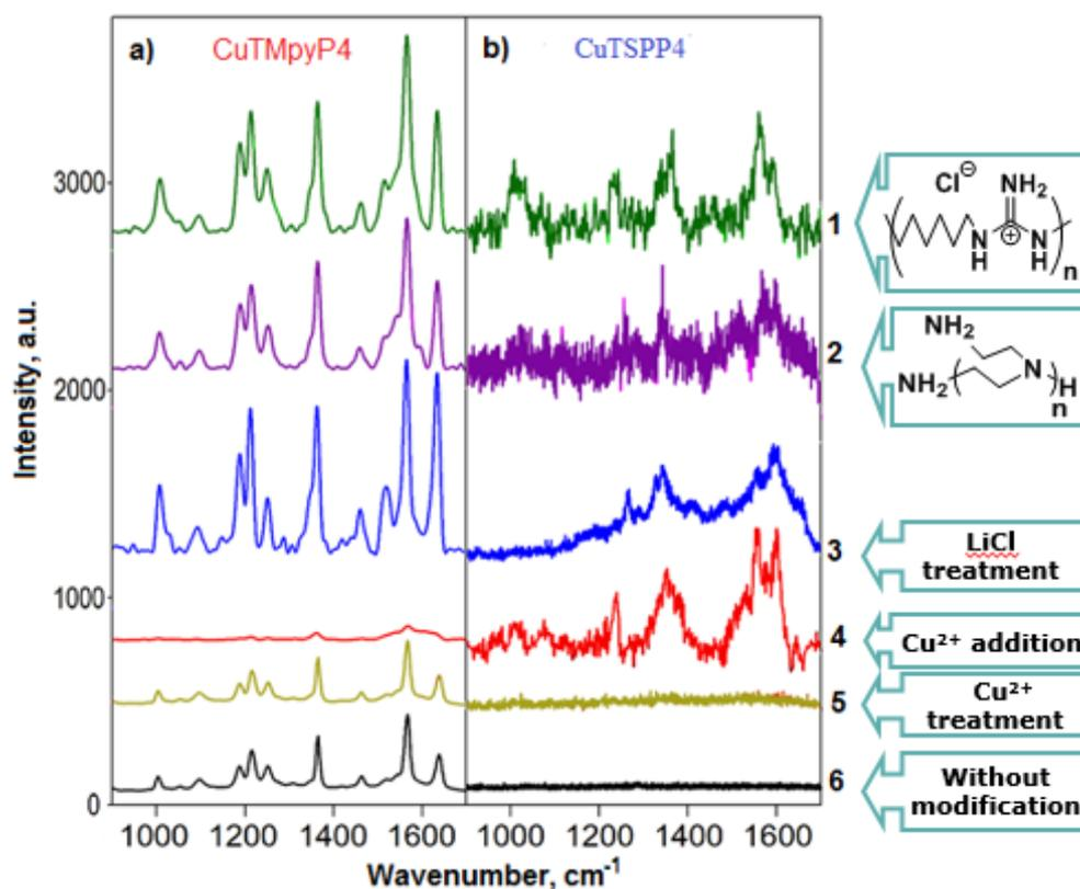
Figure 7. SERS spectra of CuTMpyP4 (a) and CuTSPP4 (b) drop-casted from  $10^{-6}$  M solution onto the SERS substrate modified with PHMG (1), PEI (2), LiCl (3),  $\text{Cu}^{2+}$  (added into analyte solution) (4),  $\text{Cu}^{2+}$  (surface treatment) (5) and unmodified plasmonic surface (6).
