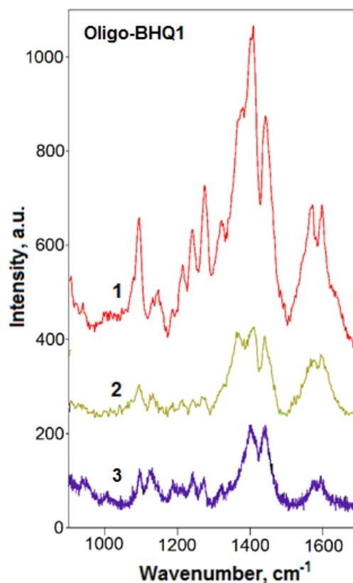
Figure 8. SERS spectra of BHQ1-labeled oligonucleotide drop-casted from  $10^{-5}$  M solution onto substrate modified with  $\text{Cu}^{2+}$  (added into the analyte solution) (1),  $\text{Cu}^{2+}$  (surface treatment) (2); Raman spectrum of BHQ1 in solution of Ag NPs (3).
