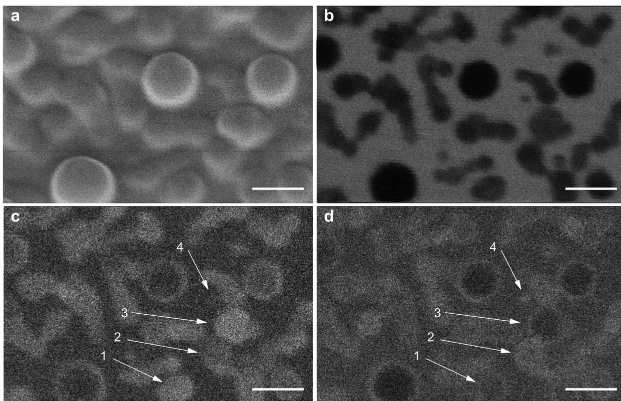
Figure 5: Thallium Chloride evaporated on a TEM grid. (a) Secondary electron image. (b) BF STIM image with acceptance angle of  $0^\circ$  to  $4^\circ$ . (c) DF STIM with polar angle from  $6^\circ$  to  $19^\circ$  and azimuthal angles  $\phi$  from  $-45^\circ$  to  $45^\circ$ . (d) DF STIM with polar angle from  $6^\circ$  to  $19^\circ$  and azimuthal angles  $\phi$  from  $135^\circ$  to  $225^\circ$ . The scale bars are 100 nm.
