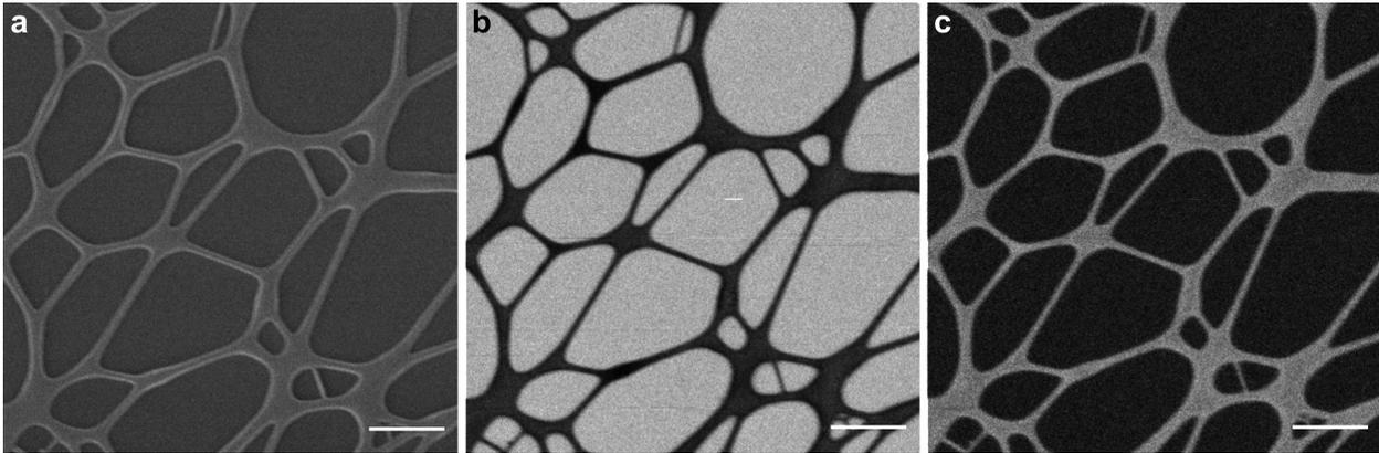
Figure 2: Micrographs of lacey carbon on carbon film in (a) secondary electron imaging mode, (b) bright field STIM image, with collection angle from  $0^\circ$  to  $3^\circ$ , and (c) annular dark field STIM image, with collection angle from  $8^\circ$  to  $13.9^\circ$ . The scale bars are  $1\ \mu\text{m}$ .
