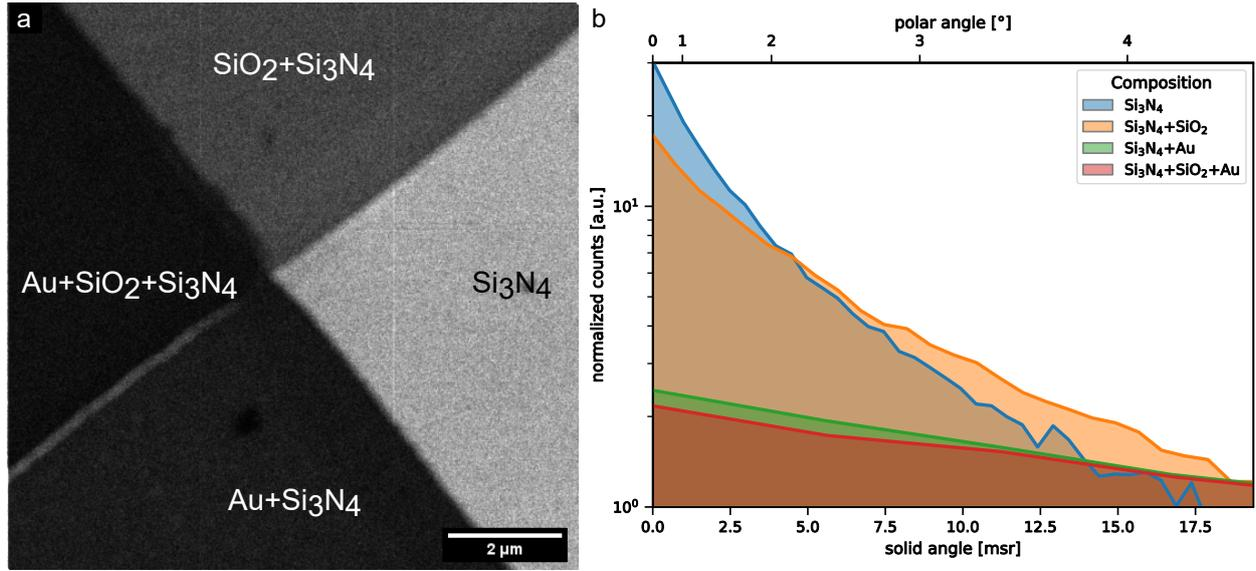
Figure 3: Bright field image showing contrast due to the exit angle dependence on the material and thickness of the layer. (a) Bright field STIM image with collection angle from  $0^\circ$  to  $4.5^\circ$  of a silicon nitride membrane with silicon dioxide deposited on the top left and gold deposited on the lower left. (b) TRIDYN simulation of the angular distribution of the transmitted beam.
