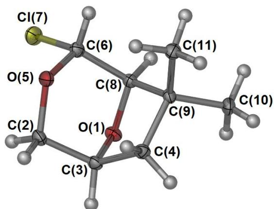
**Figure S5.** Perspective view of the labelled asymmetric unit showing the structure of **11e**, with the ellipsoids shown at 50% probability level. Carbon – grey, hydrogen – white, oxygen – red and chloride – yellow.
