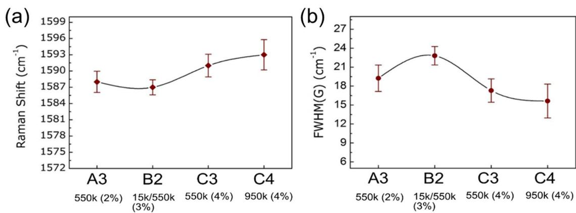
**Figure S2.** (a) Average G mode Raman shift peak position for different PMMA mixtures. (b) Average FWHM of G mode Raman shift peak for different PMMA mixtures.
