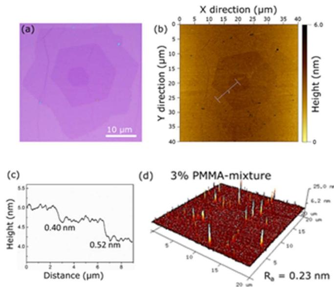
**Figure S3.** Graphene crystal transferred with B2. (a) Optical and (b) AFM image of the crystals. (c) Height profile along the white line in (b). (d) 3D surface topography ( $20 \times 20 \mu\text{m}^2$ ) and average surface roughness analysis.
