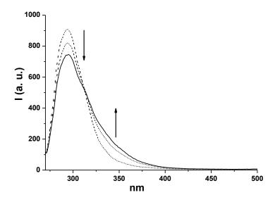
**Figure S10.** Emission spectrum of **4c** in MeOH (continuous line) and in the presence of increasing amount of 2,2,2-trifluoroethanol (up to  $20\% \text{ }_{\text{V/V}}$ , dotted line)
