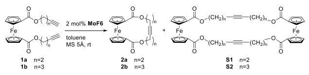
Scheme S1. Catalytic RCAM of substrates 1a and 1b towards the monomeric ferrocenophanes 2a and 2b; in some cases the formation of the dimeric ferrocenophanes S1 and S2 were observed by means of NMR spectroscopy and mass spectrometry.
