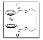
To a solution of **1a** (0.25 mmol) and MS 5Å in toluene (56 mL, 4.5 mM) the catalyst **MoF6** (2 mol%, 0.005 mmol) is added as a solid under inert Ar atmosphere. After stirring at room temperature for 2 hours the reaction mixture is filtered over silica and the patch is washed with Et<sub>2</sub>O and DCM. The orange filtrate is evaporated under reduced pressure and the crude product is purified by flash column chromatography on silica gel with 1:5 hexane/EtOAc yielding
