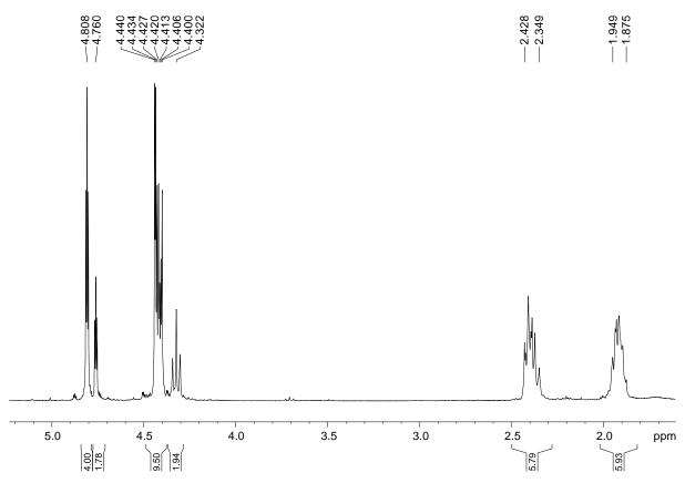
**Figure S9.** <sup>1</sup>H NMR spectrum (300.3 MHz, CDCl<sub>3</sub>, 298 K) of the crude product obtained after 4 hours from the RCAM of **1b** (0.25 mmol) with **MoF6** (2 mol%) in toluene (24 mL) in the presence of MS 5Å (500 mg), signals of desired product **2b** overlay with side product **S2**.
