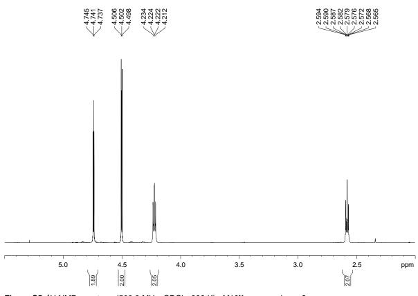
Figure S5. <sup>1</sup>H NMR spectrum (500.3 MHz, CDCl<sub>3</sub>, 298 K) of [10]ferrocenophane 2a.
