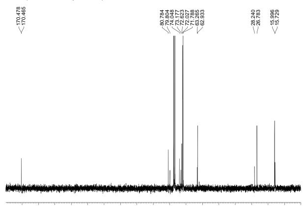
10 ppm Figure 10. <sup>13</sup>C NMR spectrum (75.5 MHz, CDCl<sub>3</sub>, 298 K) of the crude product obtained after 4 hours from the RCAM of 1b (0.25 mmol) with MoF6 (2 mol%) in toluene (24 mL) in the presence of MS 5Å (500 mg); signals of desired product 2b overlay with side product S2.
