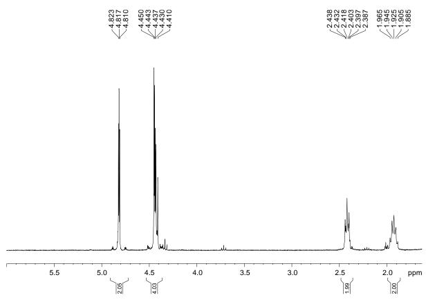
Figure S7. <sup>1</sup>H NMR spectrum (300.3 MHz, CDCl<sub>3</sub>, 298 K) of [12]ferrocenophane 2b.
