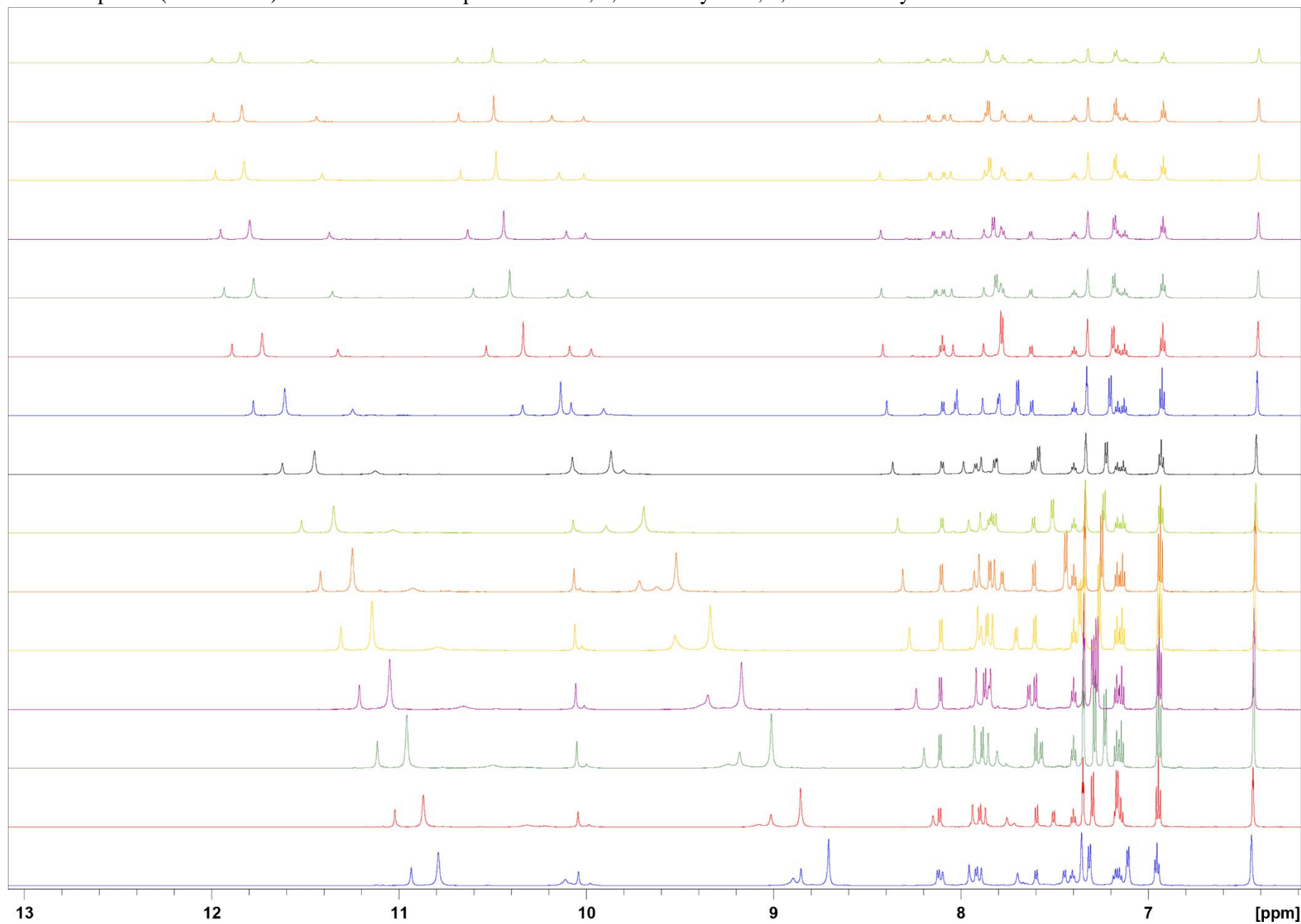
Stacked ^1\text{H} NMR spectra (700.1 MHz) of a mixture of receptors MC008 ; 1,3-diindolylurea; 1,3-dicarbazolylurea + TBA-lactate
