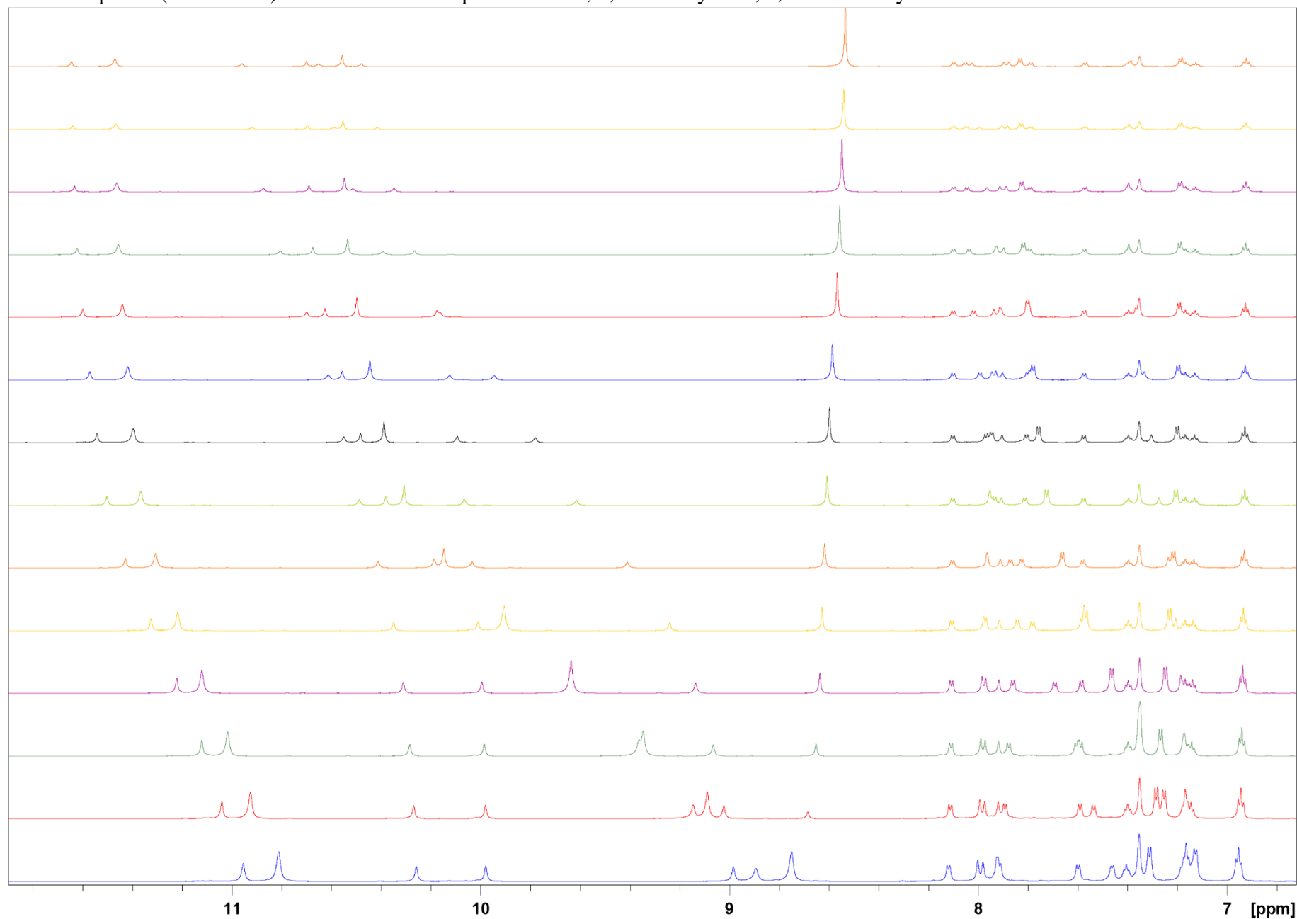
Stacked ^1\text{H} NMR spectra (700.1 MHz) of a mixture of receptors MC003 ; 1,3-diindolylurea; 1,3-dicarbazolylurea + TBA-formate
