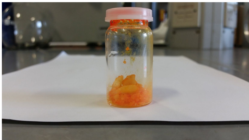
Figure 3: Clear separation of the reagents observed, with orange coated beads of 1,2-phenylenediamine residing at the bottom of the mixture.
