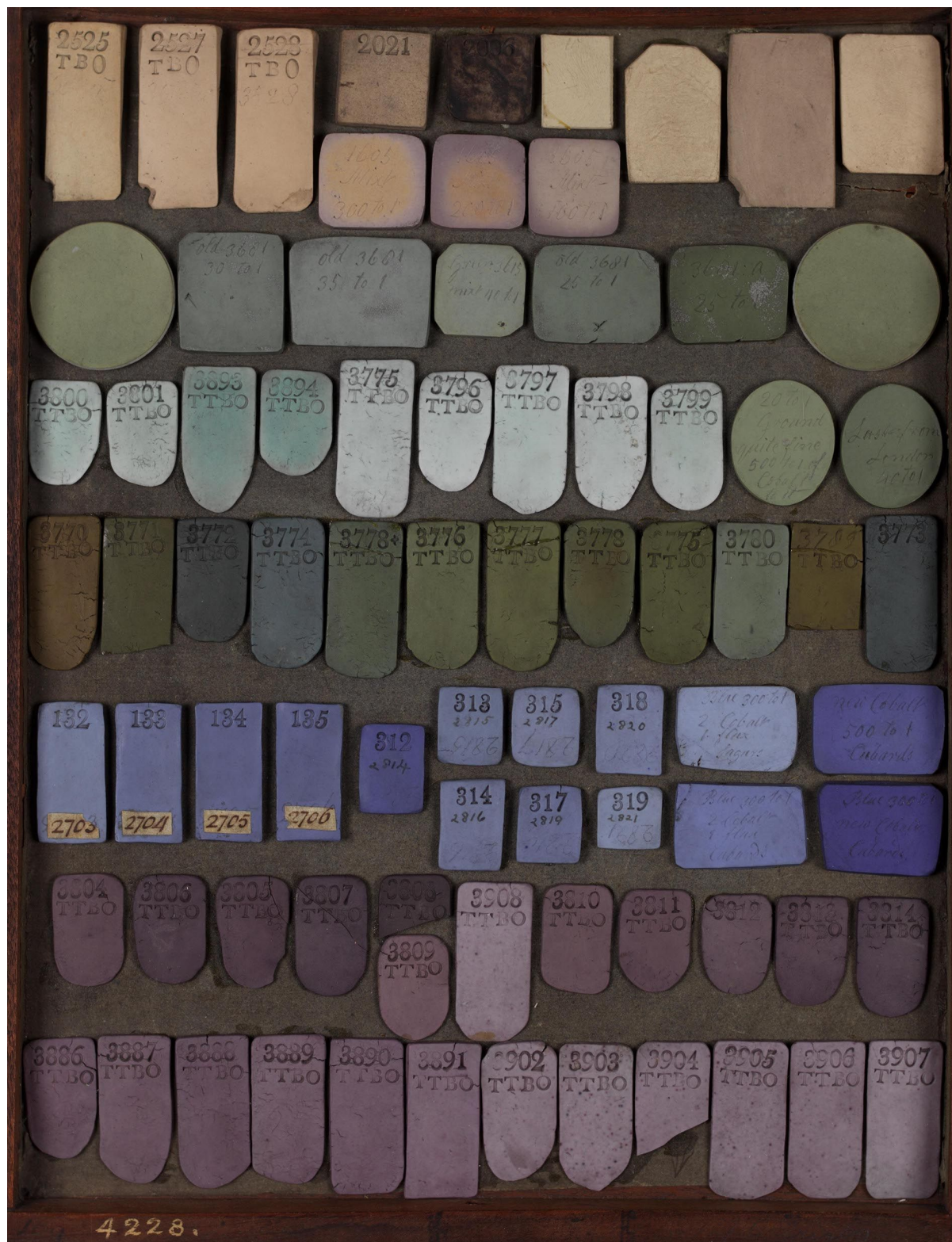
Figure 6: Tray of Josiah Wedgwood's jasper trials from 1773 (copyright Wedgwood Museum; all rights reserved). Each ceramic sample is marked with labels that correspond to an entry in Wedgwood's 'Experiment Book' or relate to firing instructions, e.g., 'TTBO' for 'tip-top of biscuit oven'. Used with permission from the Wedgwood Museum. Also see the summary of Josiah Wedgwood's work by Sammut [30].
