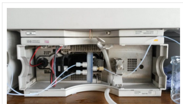
Figure 4: RD1 held in place within the DAD compartment of an Agilent 1100 HPLC.
