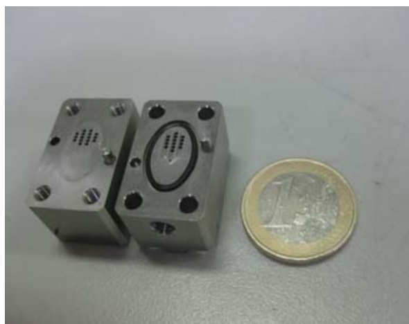
Figure 1: Hastelloy-made micromixer (MiChS \beta -150H).
