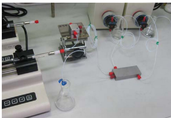
Figure 3: Acid-tolerant microflow system used for the Koch–Haaf reaction.
