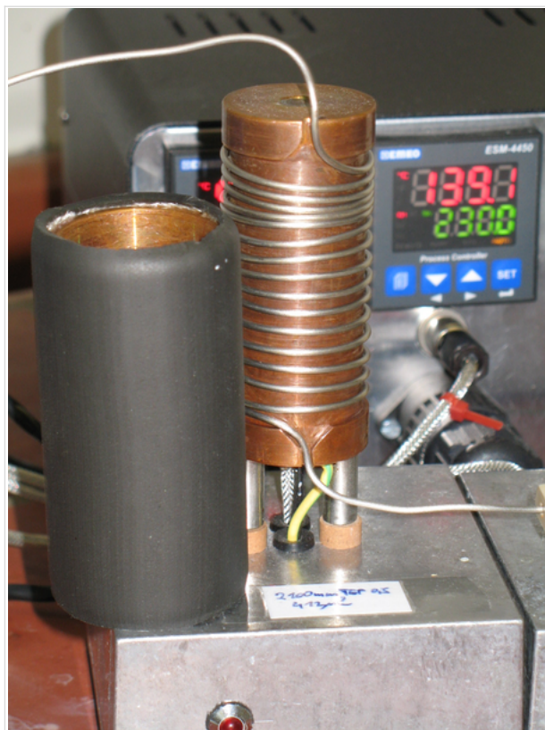
Figure 4: Capillary reactor with jacketed cover removed, and the process controller.
