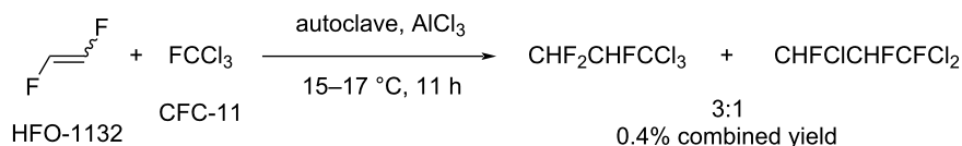
Scheme 17: Reaction of trichlorofluoromethane with 1,2-difluoroethylene.
