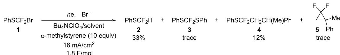
Scheme 8: Cathodic reduction of compound 1 in the presence of  $\alpha$ -methylstyrene at a high current density.Table 3: Reaction of compound 1 with SmI<sub>2</sub> in the presence and absence of  $\alpha$ -methylstyrene.
