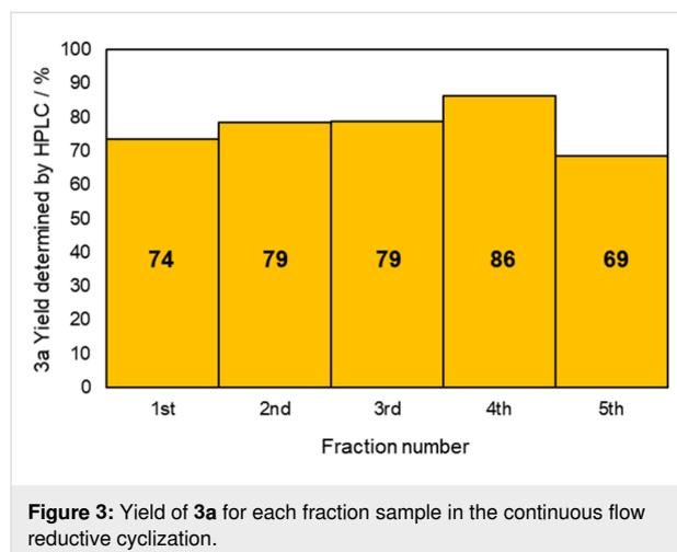
**Figure 3:** Yield of **3a** for each fraction sample in the continuous flow reductive cyclization.
