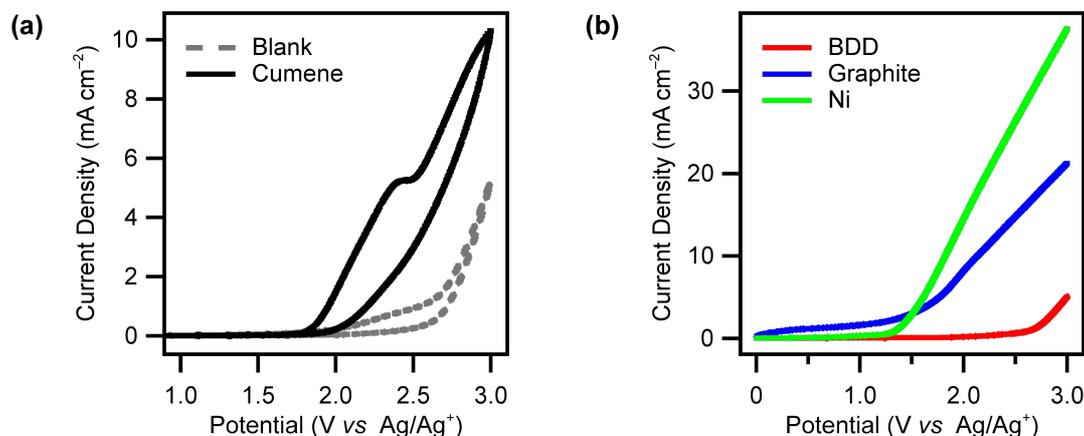
**Figure 1:** (a) Cyclic voltammograms of a BDD electrode in MeCN solution containing cumene (**1**; 5 mM) and  $\text{Et}_4\text{NClO}_4$  (0.1 M). The gray dashed line shows the voltammogram in the solution without cumene. (b) Linear sweep voltammograms of BDD (red), graphite (blue), and Ni (green) electrodes in MeCN solution containing  $\text{Et}_4\text{NClO}_4$  (0.1 M). Scan rate: 100 mV/s.
