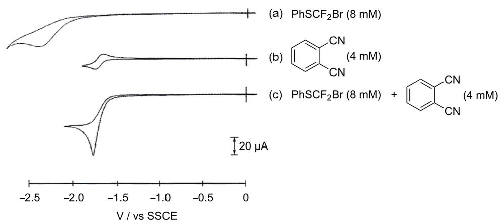
**Figure 1:** Cyclic voltammograms of (a) PhSCF<sub>2</sub>Br (1, 8 mM) in 0.1 M *n*-Bu<sub>4</sub>NClO<sub>4</sub>/MeCN; (b) *o*-phthalonitrile (4 mM), and (c) *o*-phthalonitrile (4 mM) + **1** (8 mM). Scan rate: 100 mV/s.
