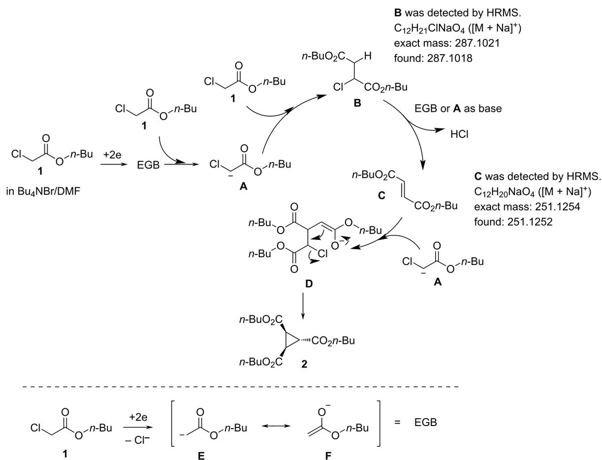
**Scheme 2:** Plausible reaction mechanism. EGB = electrogenerated base.
