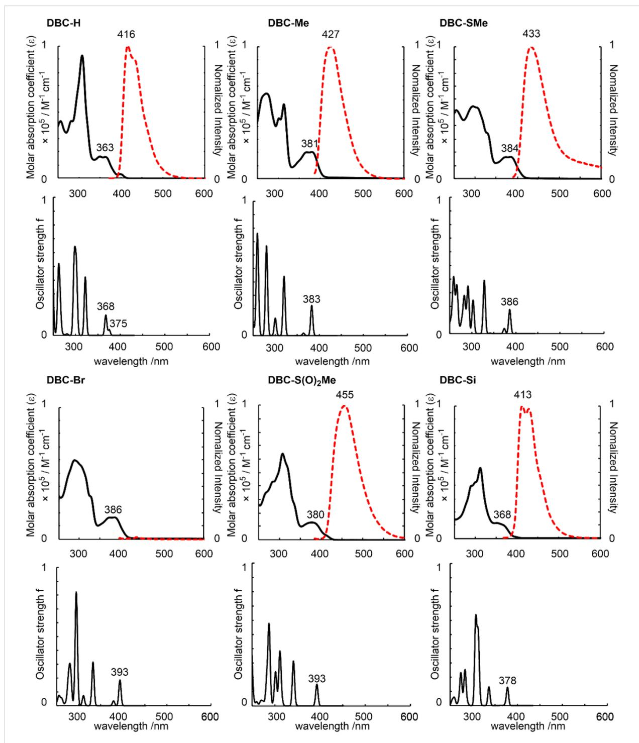
**Figure 4:** Absorption (solid line) and photoluminescence (dotted red line) spectra (upper graphs) in  $\text{CH}_2\text{Cl}_2$  and simulations of absorption based on TD-DFT calculations [lower graphs, TD-B3LYP-D3/6-31G(d,p)//B3LYP/6-31G(d,p)] for DBC derivatives.
