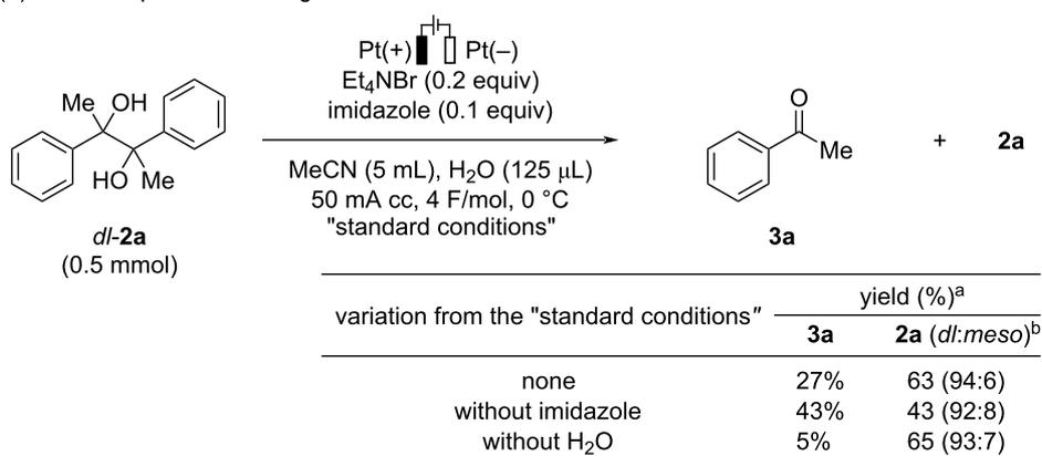
**Scheme 5:** Control experiments. <sup>a</sup>Determined by <sup>1</sup>H NMR using 1,3,5-trimethoxybenzene as an internal standard. <sup>b</sup>Determined by <sup>1</sup>H NMR analysis.
