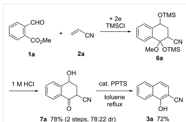
**Scheme 4:** Electroreductive coupling of **1a** with **2a** and subsequent transformation to 2-cyanonaphthalene-1-ol (**3a**).
