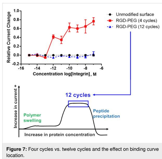
**Figure 7:** Four cycles vs. twelve cycles and the effect on binding curve location.
