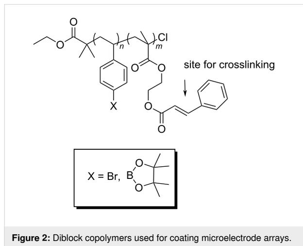
**Figure 2:** Diblock copolymers used for coating microelectrode arrays.
