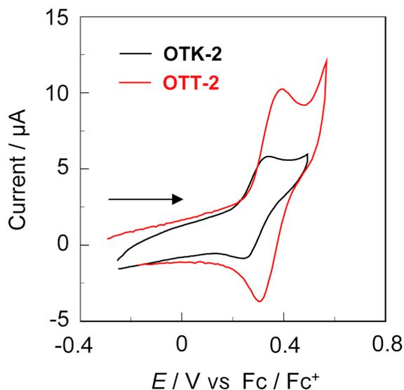
**Figure 2:** Cyclic voltammograms of **OTK-2** and **OTT-2** (0.1 mM) in DMF containing 0.1 M Bu<sub>4</sub>NClO<sub>4</sub> at a scan rate of 100 mV s<sup>−1</sup>. The arrow denotes the direction of the potential scan.
