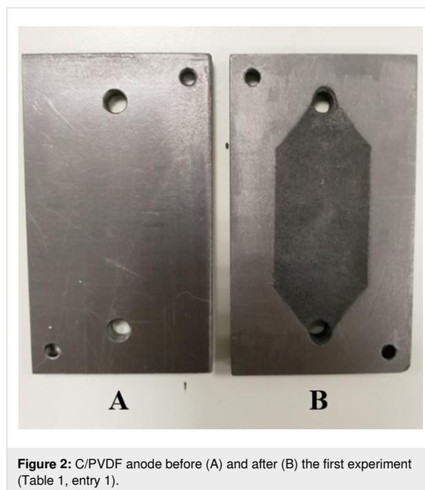
**Figure 2:** C/PVDF anode before (A) and after (B) the first experiment (Table 1, entry 1).
