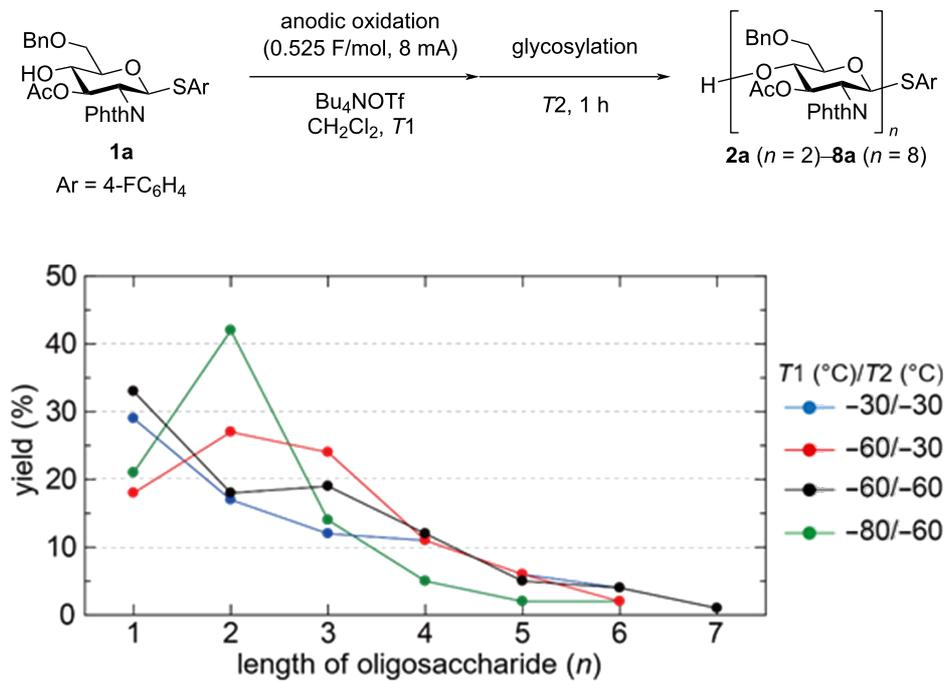
Figure 4: Influence of temperatures of anodic oxidation ( $T_1$ ) and glycosylation ( $T_2$ ).
