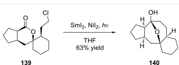
Scheme 28: Formation of variecolin intermediate 140 through a SmI 2 -mediated Barbier-type reaction.
