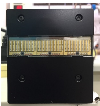
Figure 1: Components for photoflow setup: (a) MiChS LX-1 reactor and (b) MiChS LED-s (365 ± 5 nm, 60–600 W).
