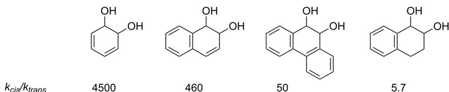
**Figure 1:** Reactivity ratios for acid-catalyzed reaction of arene dihydrodiols.
