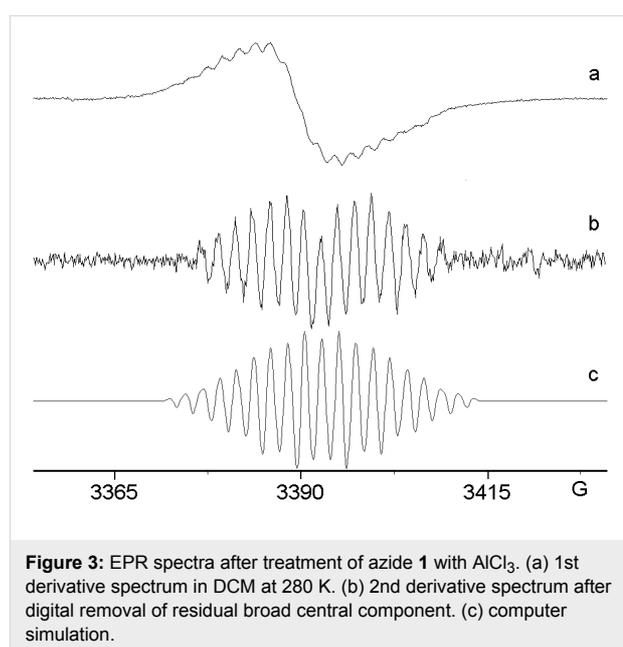
**Figure 3:** EPR spectra after treatment of azide **1** with  $AlCl_3$ . (a) 1st derivative spectrum in DCM at 280 K. (b) 2nd derivative spectrum after digital removal of residual broad central component. (c) computer simulation.
