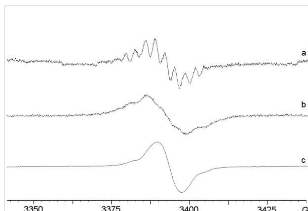
**Figure 6:** EPR spectra after In-, Ga- and Al-promoted reactions of azide **8**. (a) intermediate from  $\text{InCl}_3$  treatment of **8** at 260 K in DCM and  $\text{CH}_3\text{CN}$  (4:1). (b) spectrum from  $\text{GaCl}_3$  treatment of **8** at 300 K in DCM/pentane. (c) spectrum from  $\text{AlCl}_3$  treatment of **8** at 300 K in DCM.
