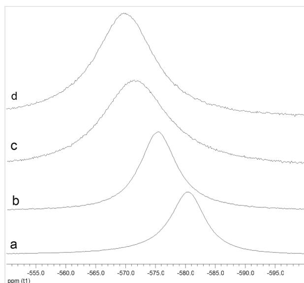
**Figure 5:** <sup>51</sup>V NMR spectra of complex **2** recorded at 50 °C. a) Spectrum in CDCl<sub>3</sub>; b) spectrum in CDCl<sub>3</sub> with 500 equiv of PhCHO added; c) spectrum in propylene carbonate; d) spectrum in propylene carbonate with 500 equiv of PhCHO added. All spectra were recorded with a complex **2** concentration of 24 mM and for spectra b and d, the concentration of benzaldehyde was 4.8 M.
