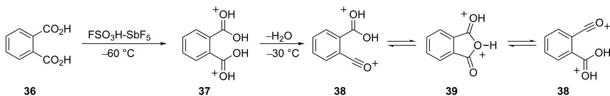
**Scheme 8:** Reaction of phthalic acid (**36**) in  $\text{FSO}_3\text{H-SbF}_5$ .
