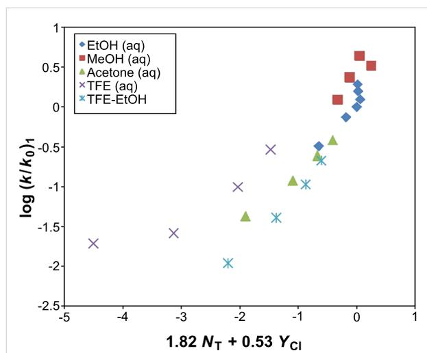
**Figure 3:** The plot of  $\log(k/k_0)$  for isobutyl chloroformate (**1**) against  $1.82 N_T + 0.53 Y_{Cl}$  in eighteen pure and binary solvents. The points for the four aqueous TFE values were not included in the correlation. They are added here to show the extent of their deviation.
