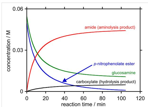
**Figure 3:** Predicted concentration-time profile for the reaction between starting concentrations of 0.05 M *p*-nitrophenyl ester **7** (R = *p*NP) and 0.055 M D-glucosamine at pH 7.41, 25 °C to 99% consumption of *p*-nitrophenyl ester **7** (R = *p*NP).
