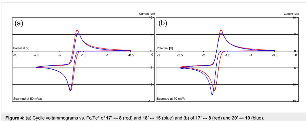
Figure 4: (a) Cyclic voltammograms vs. Fc/Fc<sup>+</sup> of **17'** ↔ **8** (red) and **18'** ↔ **15** (blue) and (b) of **17'** ↔ **8** (red) and **20'** ↔ **19** (blue).
