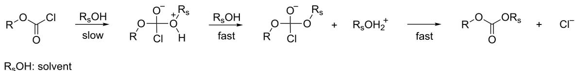
**Scheme 1:** Stepwise addition–elimination mechanism through a tetrahedral intermediate for solvolysis of chloroformate esters.
