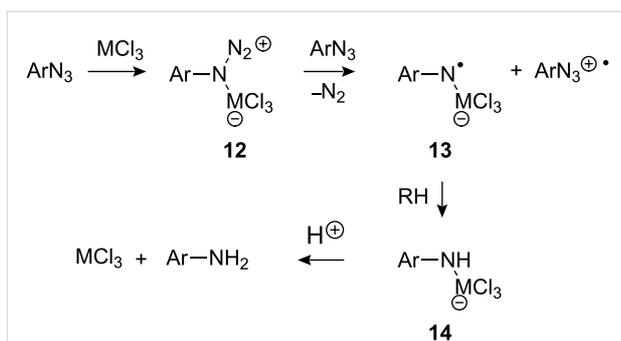
**Scheme 4:** Possible mechanism of formation of aromatic amines.
