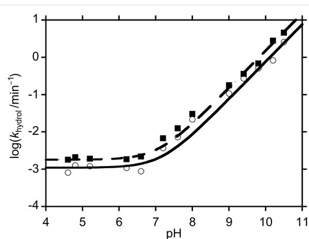
**Figure 1:**  $\log k_{\text{hydrol}}$  vs pH for the hydrolysis *p*-nitrophenyl ester **7** (R = *p*NP) and *m*-nitrophenyl ester **7** (R = *m*NP) at 25 °C. Squares correspond to data for *p*-nitrophenyl ester **7** (R = *p*NP); circles correspond to data for *m*-nitrophenyl ester **7** (R = *m*NP). The dashed line corresponds to data fitting for *p*-nitrophenyl ester **7** (R = *p*NP) and the solid line corresponds to data fitting for *m*-nitrophenyl ester **7** (R = *m*NP).
