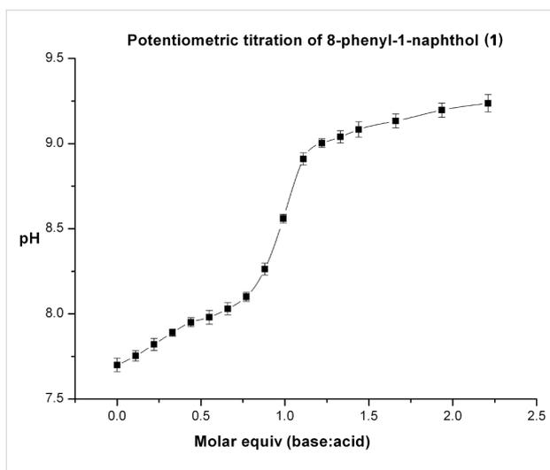
Figure 3: Potentiometric titration data for compound **1** and TBAH.
