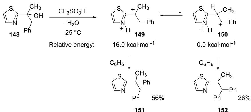
Scheme 30: Reaction of alcohol **148** in superacid with benzene.Table 3: Calculated energies of dications **153** and **154**.
