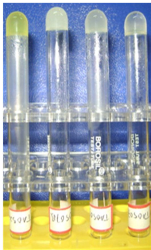
Figure 1: Photomicrographs of the organogels (from left to right: nitrobenzene gel of DBUAMC 3 ; 1,2-dichlorobenzene gel of DBAMC 6 ; chlorobenzene gel of DBAMC 6 ; bromobenzene gel of DBAMC 6 ).
